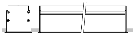
Frame recessed version / incasso con cornice variable lengths(L) x 88(W) x 87(H) mm
