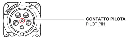
If required, the 63 A and 125 A plugs/sockets can be fitted with a pilot contact to activate an electrical interlock.
